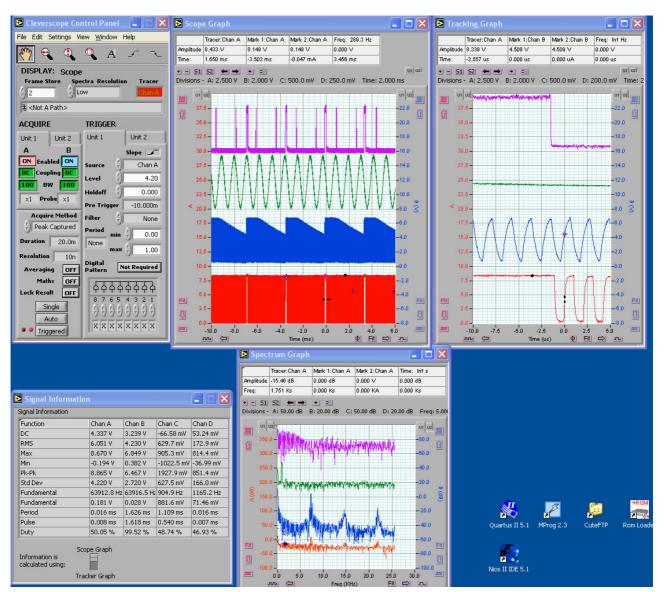
You will see that the control panel and graphs have tabs for both units. We've done it this way to make a one-to one correspondence with the physical units. You can turn on or off channels, and select coupling and BW on the Acquire Panel. You can select which unit triggers (only one unit can trigger at a time) by selecting the trigger tab, and on the tab you can select which channel triggers, and the trigger spec as normal. Dual triggers will be implemented later.
